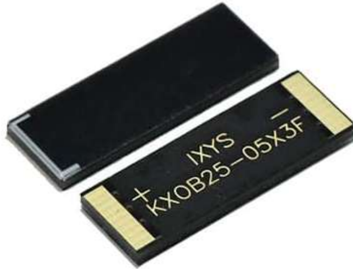
Figure 2, image of KXOB25-05X3F-TB solar cells [3].
