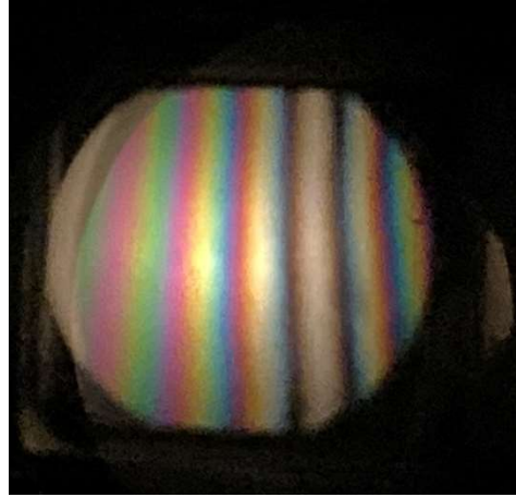
FIG. 4. The coloured fringes and the black lines of the position of zero path difference obtained with white light.
