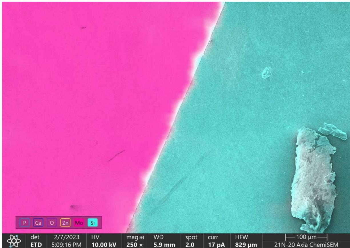
Figure 4-5: EDS map of the junction in the wafer, silicon is blue and molybdenum is pink. The boundary between the materials is shown and aligns with the line seen in SE images. In the bottom right corner, a piece of dust is on the sample (Nancy Van Wagoner).
